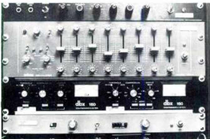
Figure 5. An Orban 672A "Paragraphic" equalizer, with typical "phoner-fix" settings shown. The settings are approximately 55 Hz/0 dB, 120 Hz/0 dB, 150 Hz/+5 dB, 400 Hz/-7 dB, 600 Hz/-4 dB, 2.5 kHz/+4 dB, 4.5 kHz/0 dB, 5 kHz/-1 dB. The high- and low-pass filters on this unit are not as steep as on the UREI "Little Dipper," which is used for this purpose and is inserted ahead of the Orban equalizer. The dbx 160 compressor gives good results with phoners. (Photos by Skip Pizzi.)
